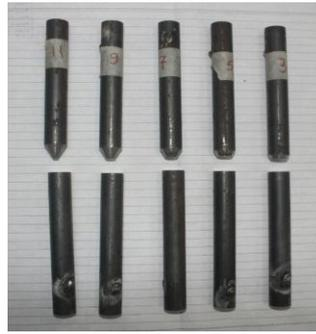
Figure 2.2 Specimen before Welding Run
